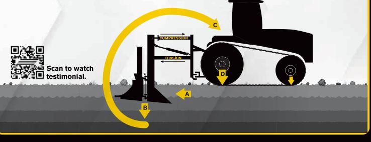
The Tile PRO Plow achieves active weight transfer through the use of a quick-attach mounting system that bolts on to the tractor frame. This maximizes traction by distributing plow draft force evenly across the tractor frame for optimum performance in all conditions.
